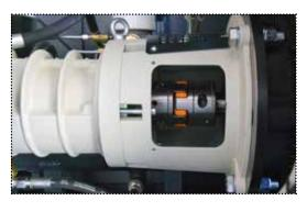
BLADE 8-12 i has been designed in a way that makes it possible **to replace the elastic element** without having to dismantle the rotor-stator unit.
